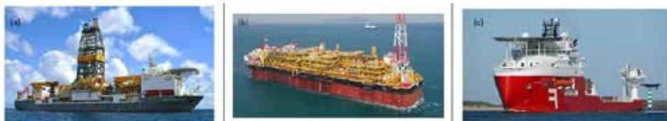
Figure 1 : (a) Rig de forage Rowan Renaissance. (b) FPSO Pazflor. (c) FSV Far Sleipner
