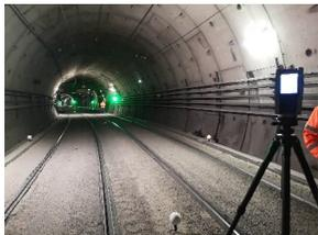
Figure 1 : Acquisition scanner laser terrestre
