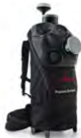
Figure 1 : Pegasus Backpack de Leica
