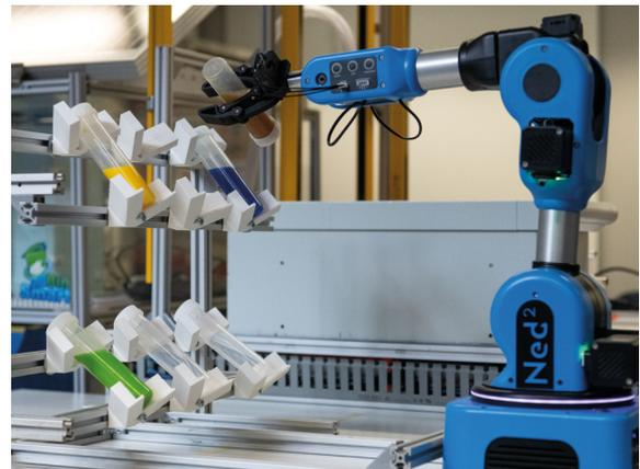
Bras robot programmable 6 axes
